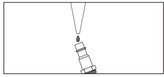
Figure 3. Lubricating directly into air fitting.
